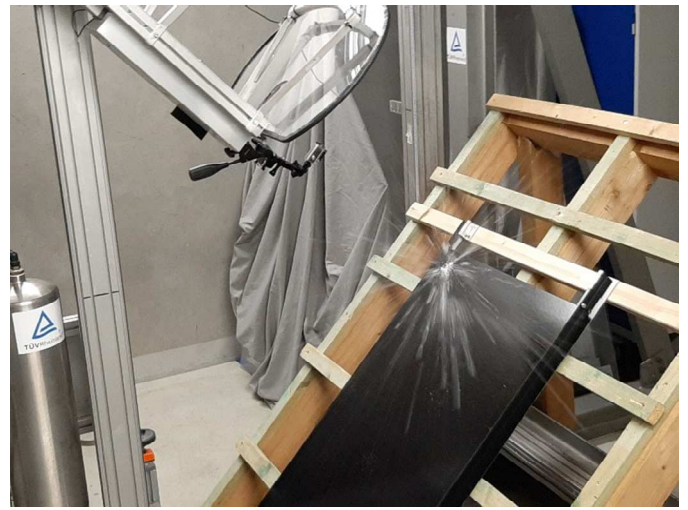
Example of Impacts on Corner VKF (40 mm)
