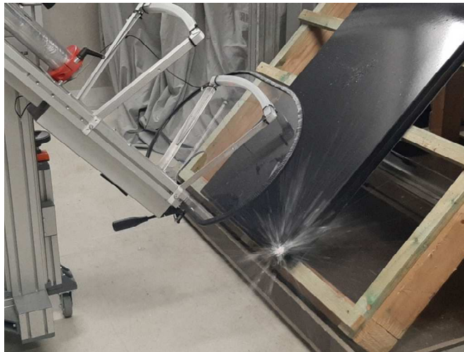
Example of Impacts on Corner ADD (40 mm)
