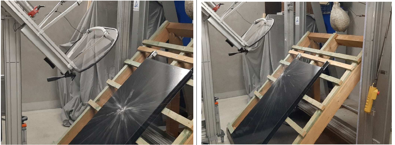
Example of Impacts on Corner ADD (40 mm)
