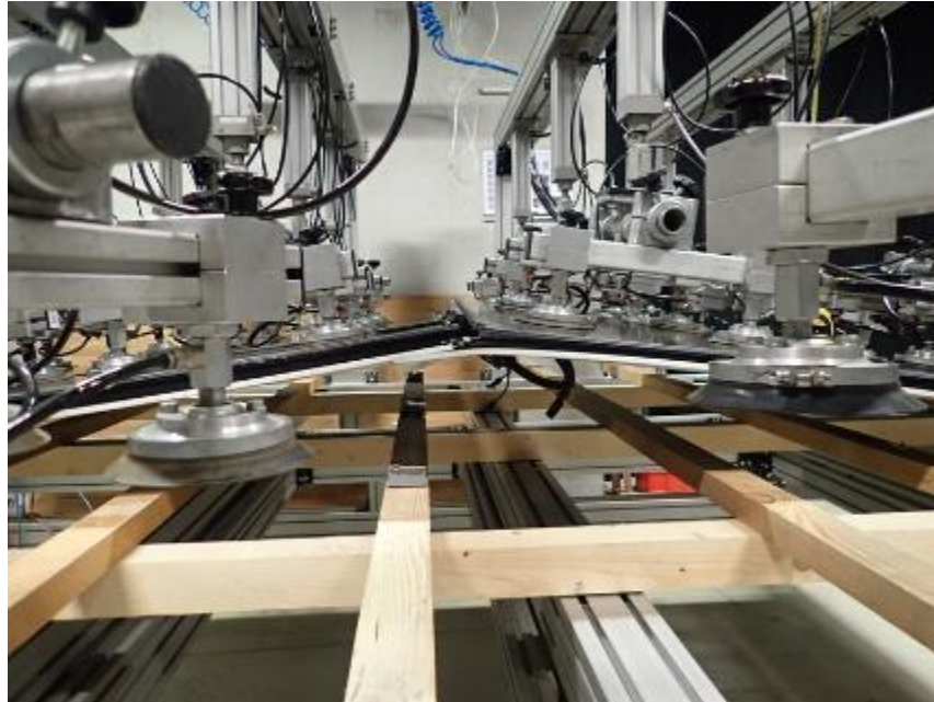
Fig. 15: failure second test at 2750 Pa
