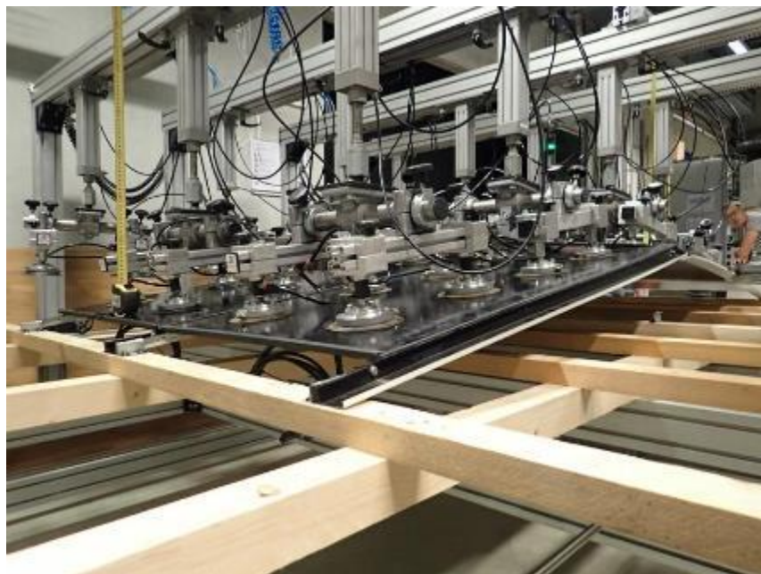
Fig. 16: failure second test at 2750 Pa
