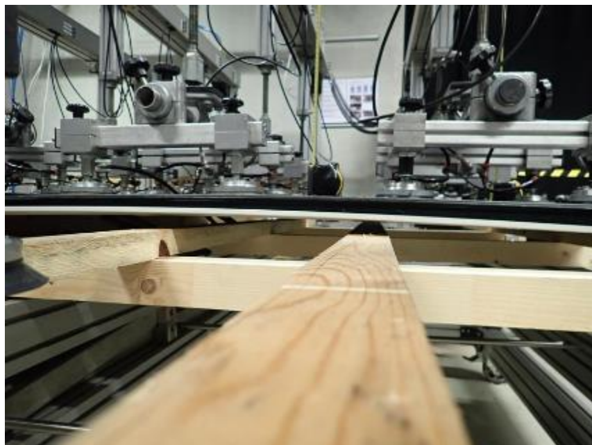
Fig. 8: system while testing at 2500 Pa
