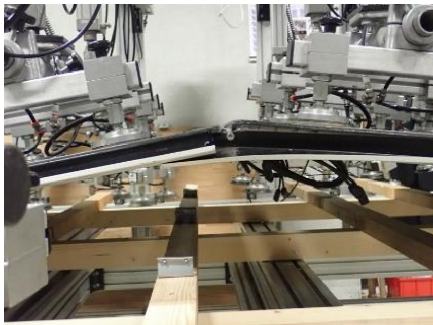
Fig. 12: failure first test at 2750 Pa
