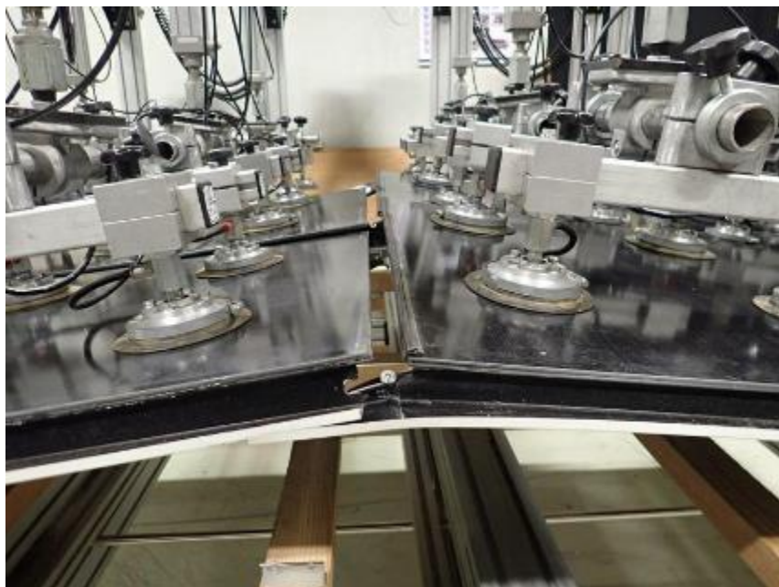
Fig. 18: failure second test at 2750 Pa
