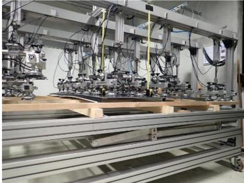
Fig. 7: system while testing at 2500 Pa
