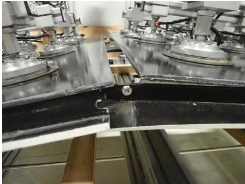
Fig. 13: failure first test at 2750 Pa
