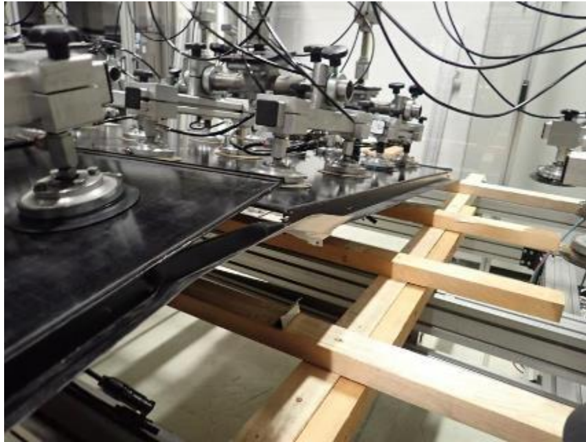
Fig. 17: failure second test at 2750 Pa
